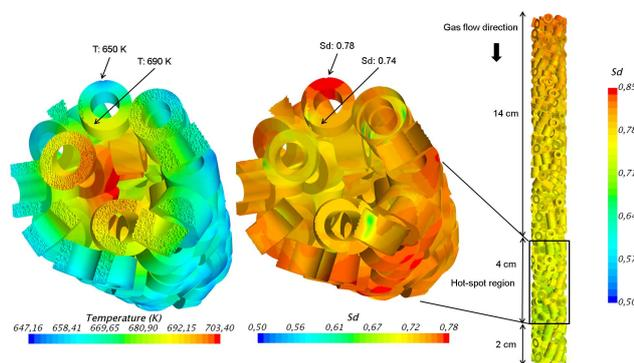
Fig. 2 Particle Resolved CFD Simulation of Temperature and Differential Selectivity in a Fixed-Bed Reactor for n-Butane Oxidation to Maleic Anhydride on a Vanadyl Pyrophosphate Catalyst.
